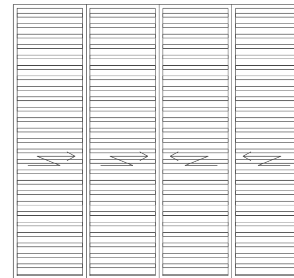
TYPICAL ELEVATION - BALCONY SCREEN
